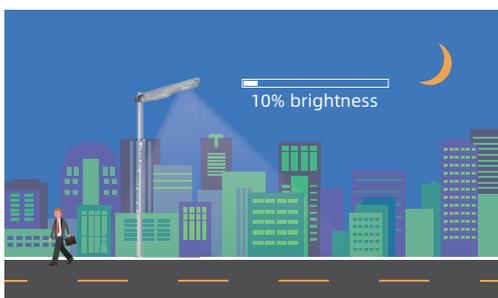
The light keeps 10% brightness when there is no presence detected.
