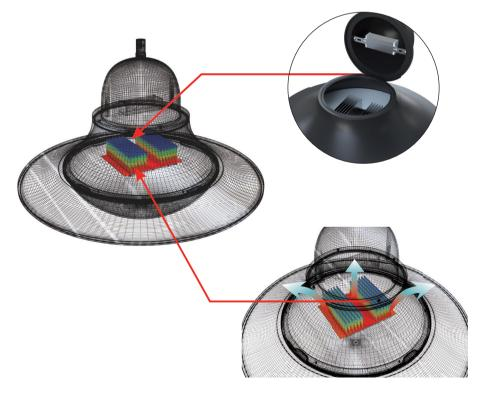
Non-contact structure for LED drivers and heat sinkers. The electrical parts are in cool status.
